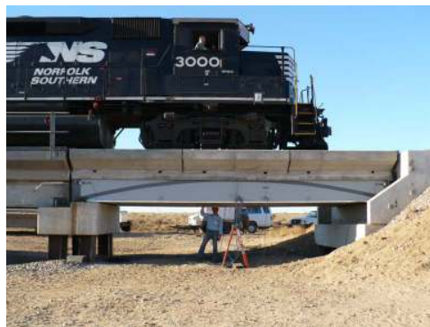
Live Load Tests on Prototype HCB Bridge
