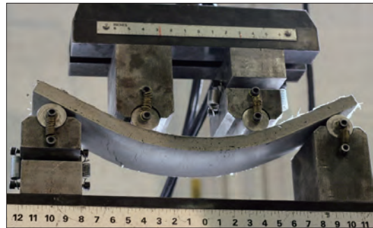
(b) Ductile failure of ECC
